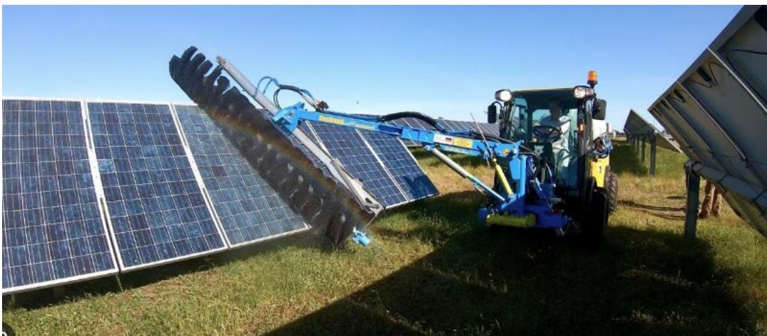
Photo 48: Cleaning of Solar Arrays
