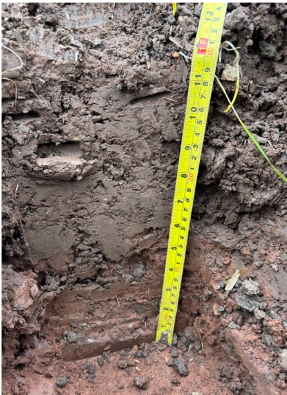
Photos 8 and 9: Subgrade 3b in Parcel 244, reddish clayey soils over mudstone
