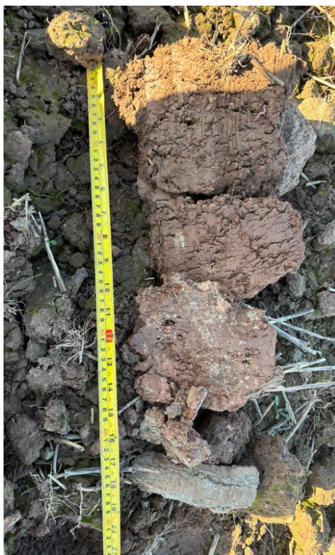
Photos 4 and 5: Subgrade 3a in Parcel 79, reddish fine loamy soils
