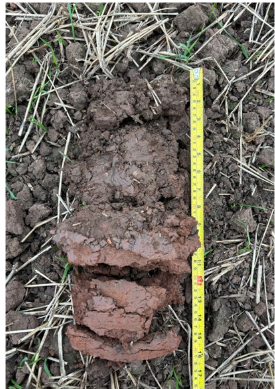
Photos 8 and 9: Subgrade 3b in Parcel 244, reddish clayey soils over mudstone
