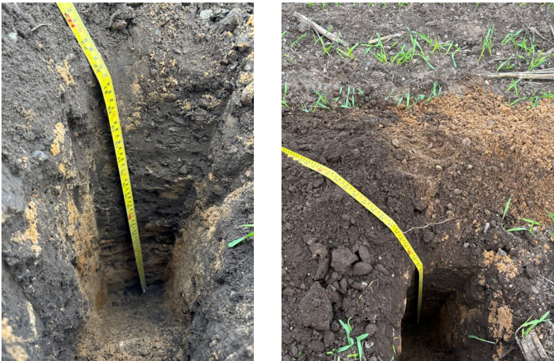
Photos 18 and 19: Pit and soils showing clear colour distinction
